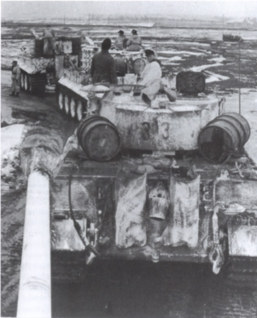
A column of late-production Tiger Is on the Eastern Front. Even though its crews considered it invulnerable, Guderian noted in October 1943 that it could be destroyed by the Soviet 76.2mm gun at a range of 500m, while its bulk attracted massive enemy fire, even from the artillery. (Private collection)
